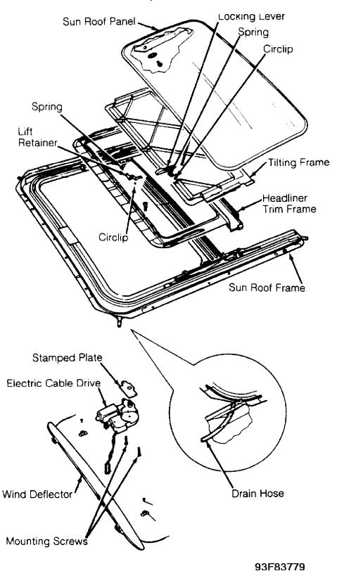
Fig. 5: Exploded View Of Power Sun Roof Assembly (Corrado SLC & Passat)
